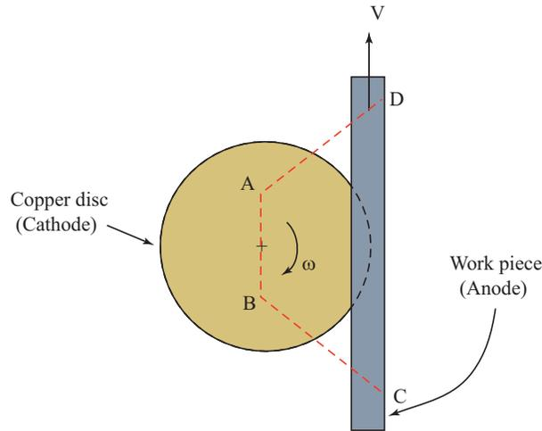
Fig. 4 Schematic sketch of the arc ablation process for developing a mathematical model. The computational domain ABCD is fixed in space, and material flows through it.
