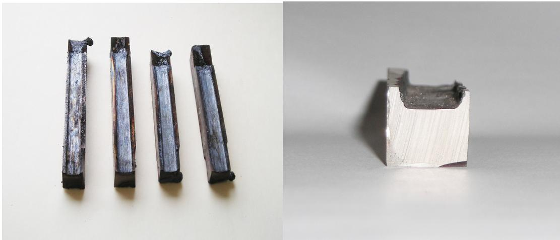
Figure 2. Four HSS test pieces 12mm wide. Figure 3. Sample #11: grooved HSS test piece
