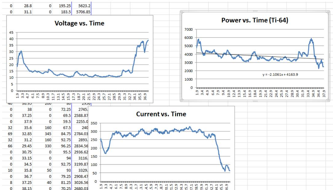
Figure 5. Electrical Measurements during a Ti-64 Grooving Experiment.
