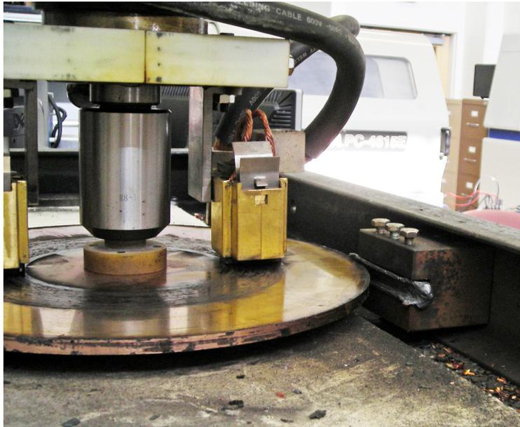
Figure 1. Experimental set-up with copper disk and high speed steel work piece.
